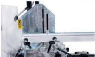
1 dikey 2 yatay mengene sistemi 1 vertical 2 horizontal vise system
